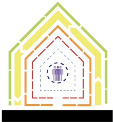
Above: the 7 layers of buildings: site, structure, skin, services, space plan, stuff, social
